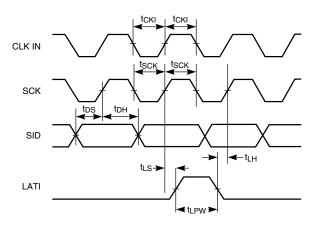
Figure 1. Serial Interface Timing.
