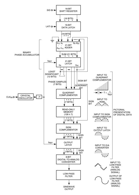
Figure 4. Detailed Block Diagram of the ML2036
