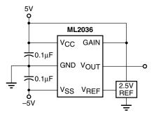
Figure 8. Sine Wave Generator with ± 2.5VP-P.
