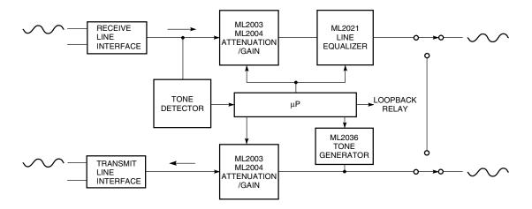
Figure 7. 4-Wire Termination Equipment.
